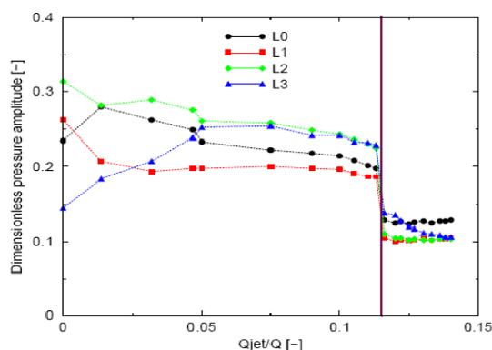
Fig.2 The sudden drop of pressure amplitude starting with 11.5% from the main discharge, jet injection [3].
