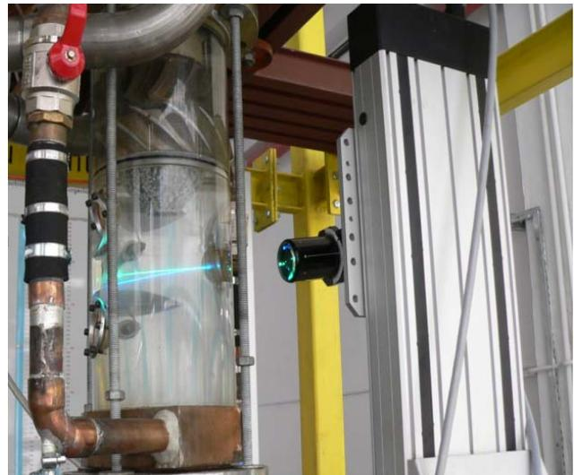
Fig.9 LDV system during the velocity profiles measurements.
