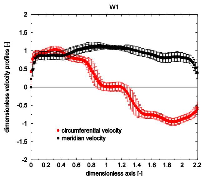
Fig.13 The velocity profiles for the case with flow-feedback jet injection method, with nominal flow at 25.5 and 30 l/s.
