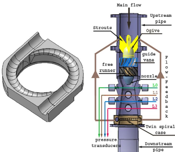
Fig.5 Spiral case with double exit (left), and cross-section of the assembled test section with twin spiral case (right).
