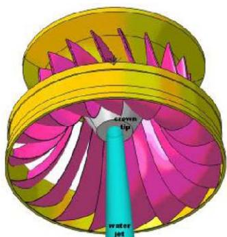
Fig.1 Water jet injection along the runner crown.
