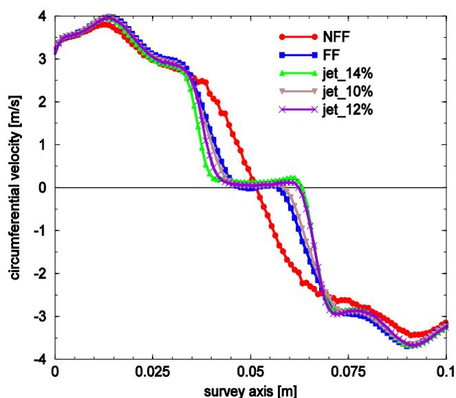
Fig.11 Circumferential velocity profiles.
