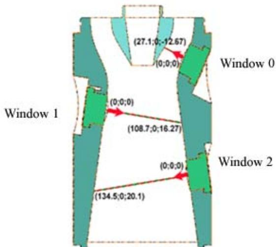
Fig.8 Test section with the three optical windows and the corresponding survey axis for measuring the velocity profiles.
