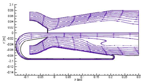
Fig.3 Streamlines for the axisymmetric swirling flow without flow control (upper half-plane) and with flow-feedback control (lower half-plane) [12].
