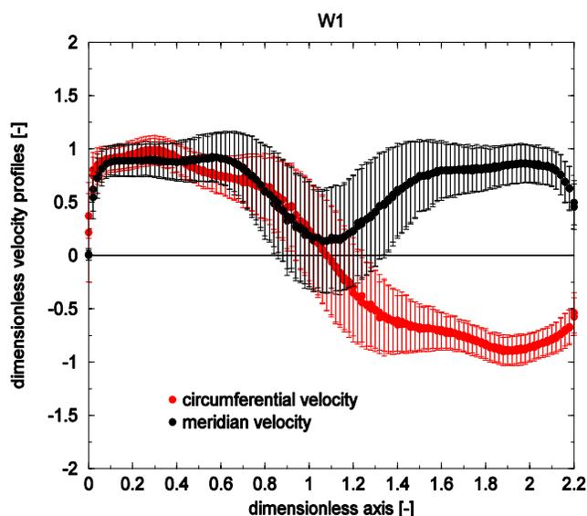
Fig.12 The velocity profiles for the case without flow-feedback jet injection method, with nominal flow at 25.5 and 30 l/s.
