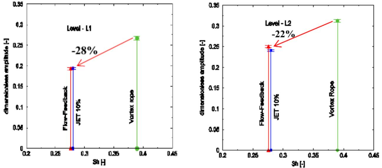
Fig.7 Comparison of the two jet injection methods and the case without jet injection method respectively, in terms of dimensionless amplitude vs. Strouhal number.
