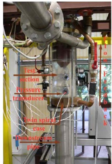
Fig.6 Implementing of flow-feedback technique on the test rig.
