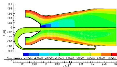
Fig.4 Total pressure for the axisymmetric swirling flow without flow control (upper half-plane) and with flow-feedback control (lower half-plane) [12].
