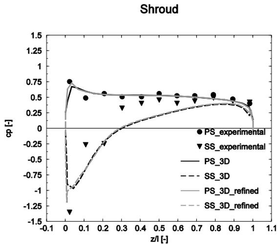
**Figure 9. Pressure coefficient distribution along the inducer blade, at radius  $r = 0.145$  m, for the 3D domain**
