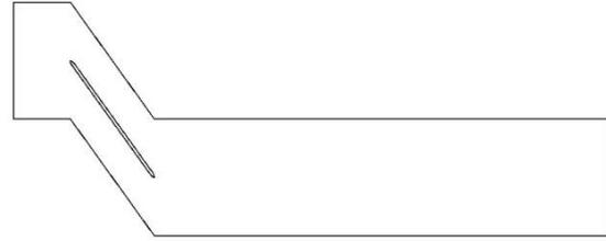
**Figure 3. 2D computational domain of the inducer**
