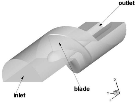
**Figure 4. 3D computational domain of the inducer**
