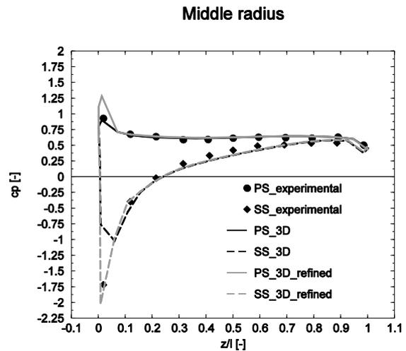
**Figure 7. Pressure coefficient distribution along the inducer blade, at radius  $r = 0.111$  m, for the 3D domain**
