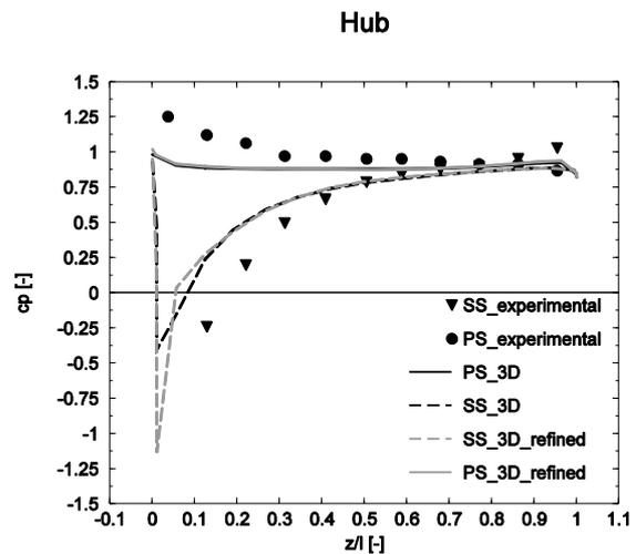
**Figure 8. Pressure coefficient distribution along the inducer blade, at radius  $r = 0.05$  m, for the 3D domain**
