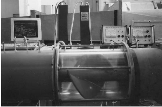
**Figure 2. Test rig for pressure measurement on the blade of an inducer**
