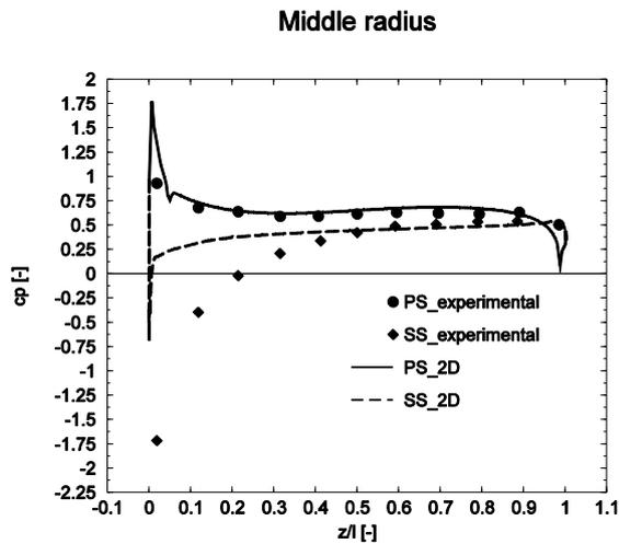
**Figure 5. Pressure coefficient distribution along the blade of the inducer, at the middle radius, for 2D domain**
