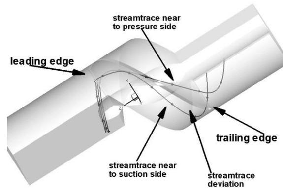
**Figure 11. 3D deviation of the stream trace on the suction side**
