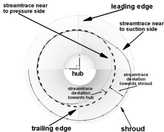
**Figure 10. 3D effects on the loading of the inducer blade for stream trace positioned at  $r = 0.111$  m**
