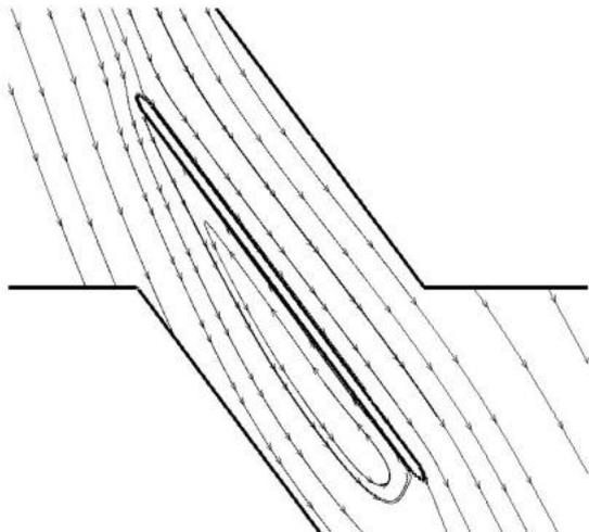
**Figure 6. Distribution of the streamlines, at the middle radius, for 2D domain**
