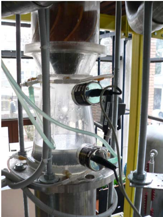
Fig. 4. Pressure transducers already mounted on the test section
