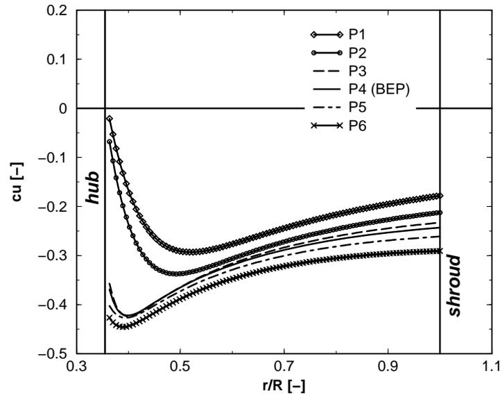
**Figure 8. The distribution of the tangential velocity coefficient versus dimensionless radius upstream the Kaplan runner for operating points.**
