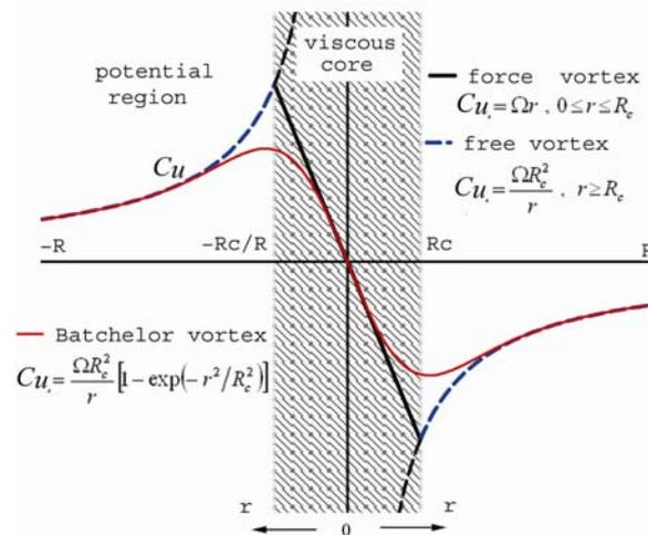
**Figure 4 The models of tangential velocity distribution in swirling flow.**
