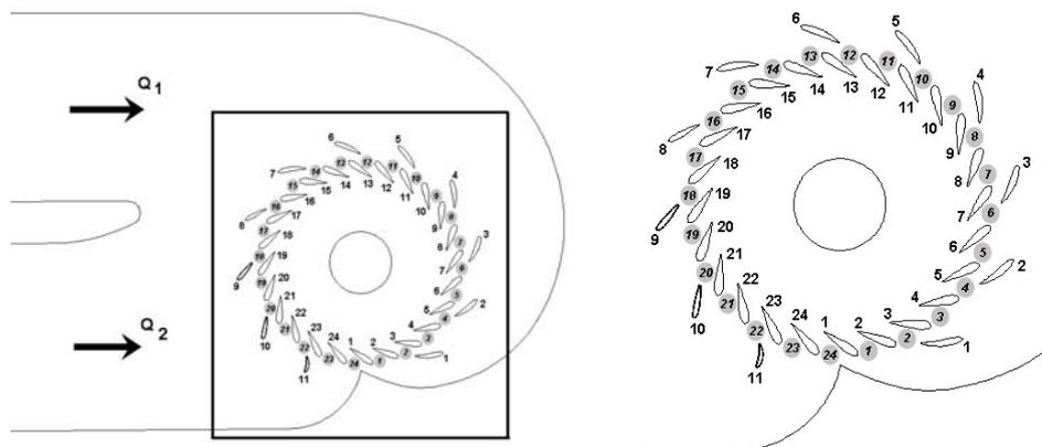
**Figure 2 Top view of the spiral case and distributor (left) and a detail view of the stay and guide vanes (right).**
