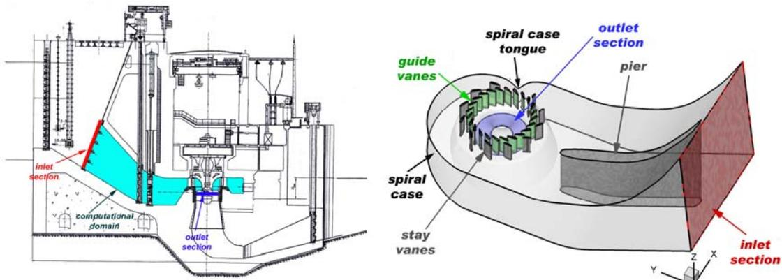
**Figure 1 3D computational domain extends from the power plant inlet to the runner reference plane.**
