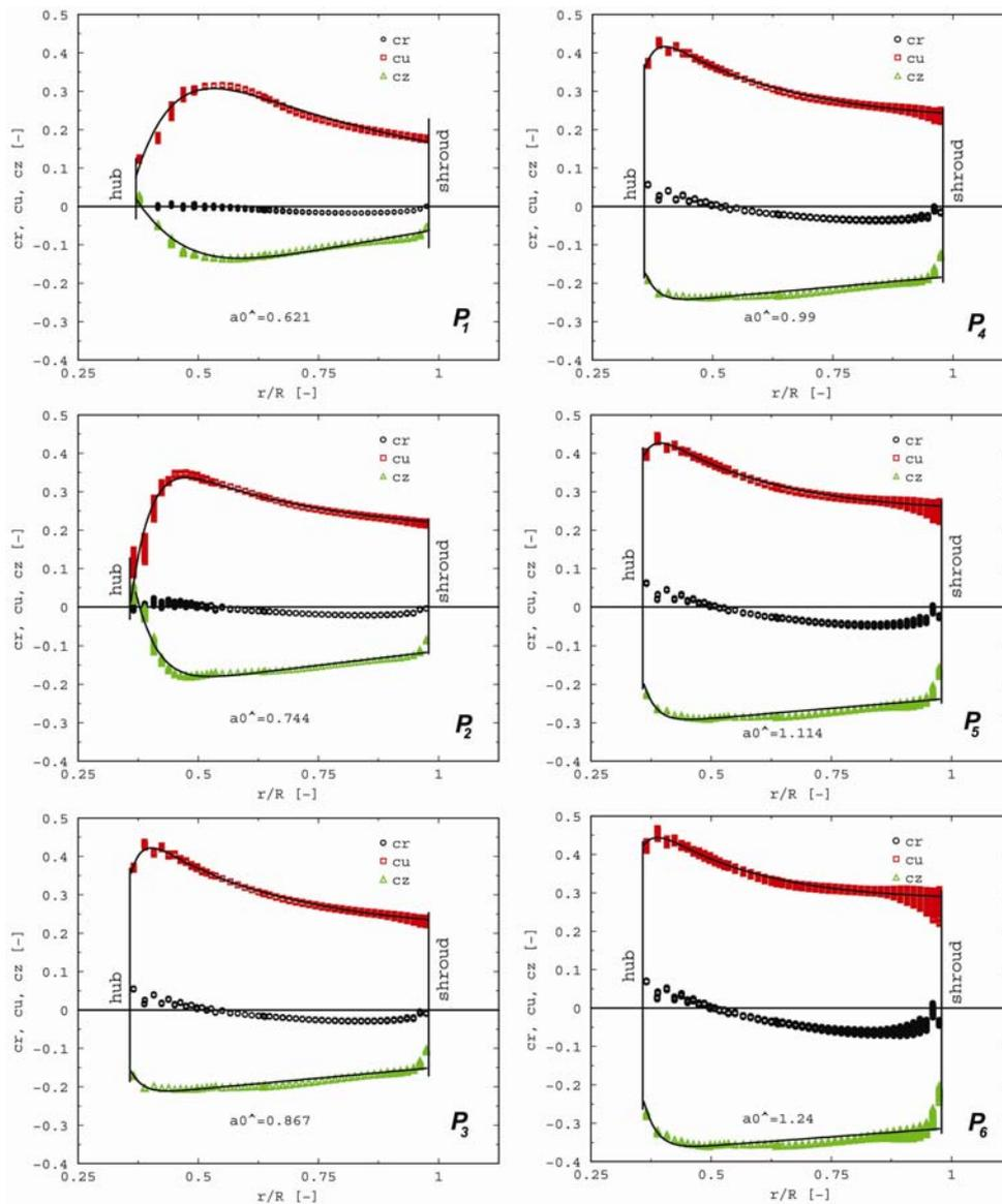
**Figure 5 The velocity coefficients versus dimensionless radius upstream the Kaplan runner for operating points investigated.**
