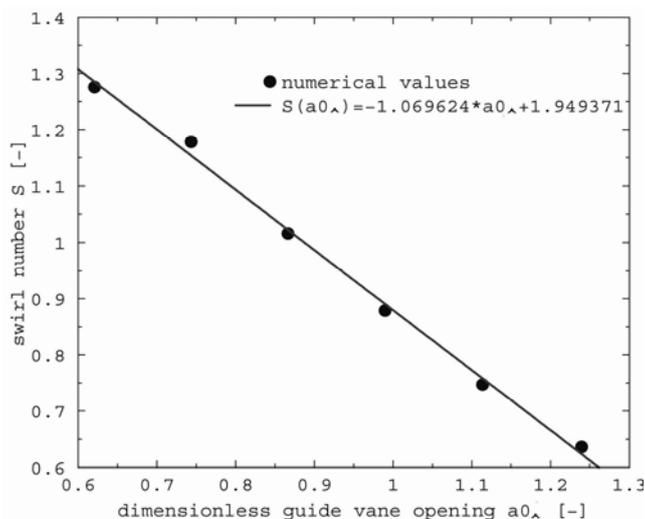
**Figure 9. The swirl number versus dimensionless guide vane opening.**
