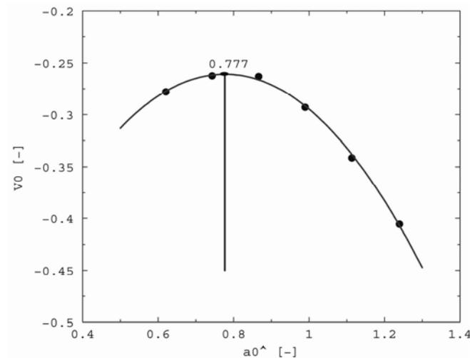
**Figure 7. The distribution of the characteristic velocity of solid body vortex versus dimensionless guide vane opening.**
