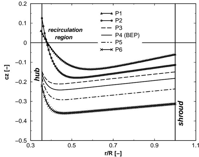
**Figure 6. The distribution of the axial velocity coefficient versus dimensionless radius upstream the Kaplan runner for operating points.**
