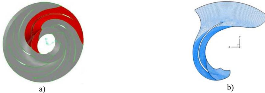
**Fig. 1** a) Impeller of the storage pump with highlighted inter blade channel
