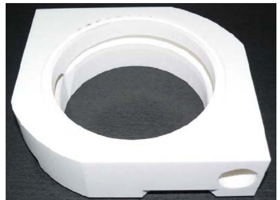
Fig. 5 Twin spiral case manufactured by rapid-prototyping machine.
