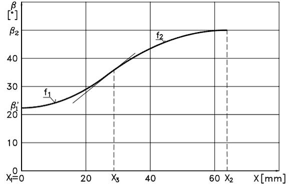
Fig.1  $\beta$  interpolation with two parabola arcs direct connected
