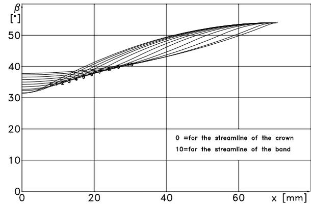
Fig. 3. Distribution of relative flow angle  $\beta$  on streamlines for the impeller with  $n_q=18.18$
