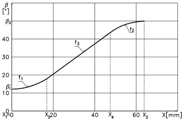
Fig. 2. Relative flow angle  $\beta$  interpolation with two parabola arcs connected by a straight segment line
