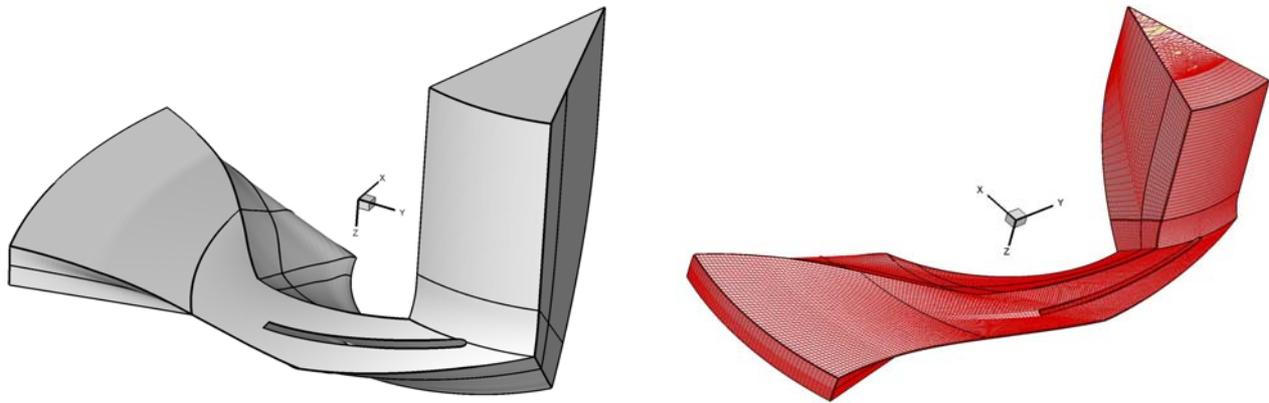
Fig. 11. 3D computational domain and mesh on the channel of the impeller with  $n_q=100.26$
