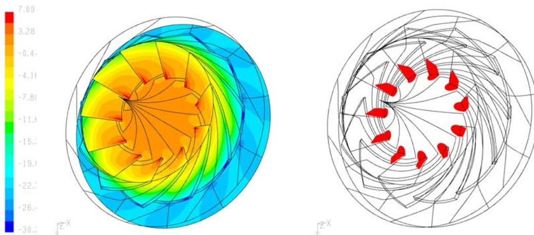
Figure 14. NPSH<sub>r</sub> distribution on the impeller with  $n_q=100.26$  (left). The red spots indicate maximum risk at cavitation development (right).
