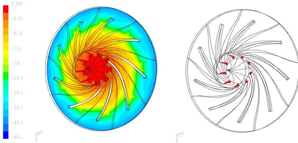
Figure 12. NPSH<sub>r</sub> distribution on the impeller with  $n_q=18.18$  (left). The red spots indicate maximum risk at cavitation development (right).
