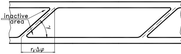
Fig. 4. Lean angle of the blade impeller at the outlet.
