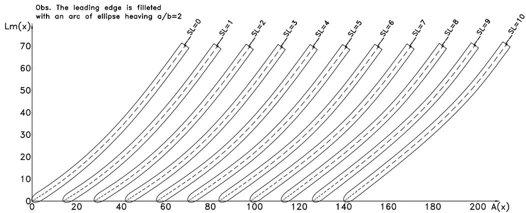
Fig. 7. The streamlines and their hydrodynamic profiles in the conformal mapping plan for all sections for the impeller with  $n_q=18.18$
