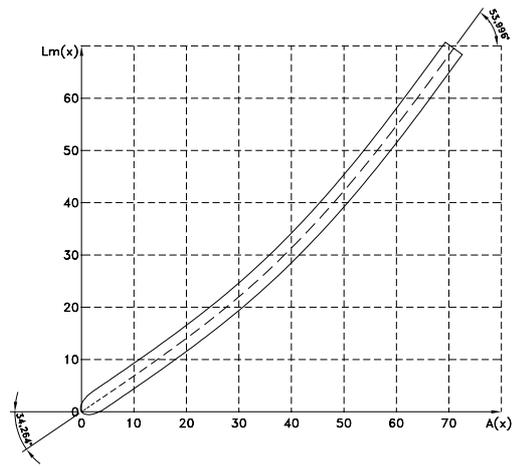
Fig. 6. The profile of the blade of constant thickness in the conformal mapping plane
