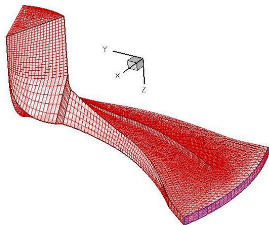
Fig. 9. 3D computational domain and mesh on the channel of the impeller with  $n_q=18.18$
