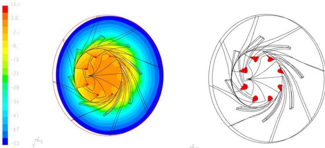
Figure 13. NPSH<sub>r</sub> distribution on the impeller with  $n_q=47.50$  (left). The red spots indicate maximum risk at cavitation development (right).
