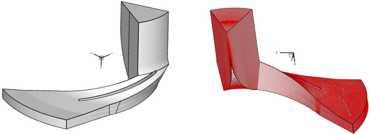
Fig. 10. 3D computational domain and mesh on the channel of the impeller with  $n_q=47.50$
