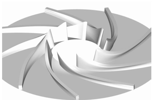
Fig. 8. 3D image of the impeller blades (the band surface was removed)
