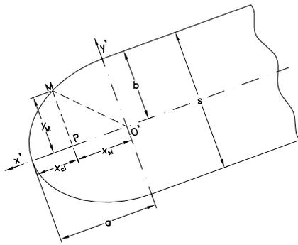
Fig. 5. Leading edge profile with ellipse arcs
