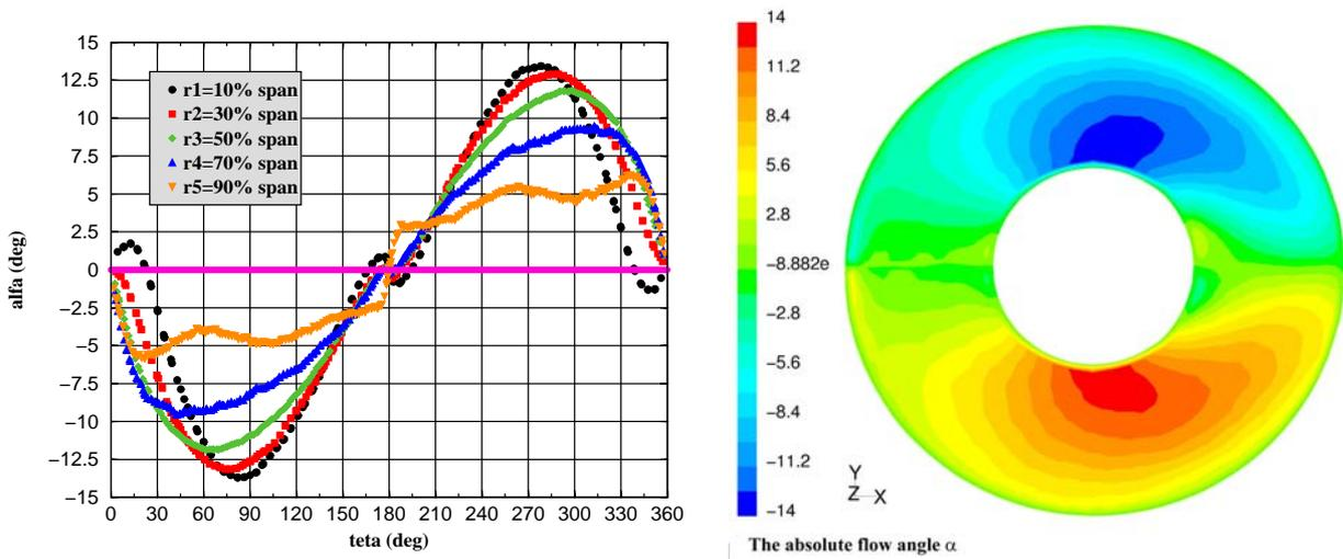
Figure 14. The absolute flow angle ( $\alpha$ ) distribution on the outlet section of the suction domain
