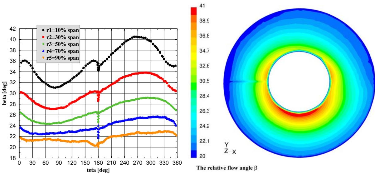
Figure 15. The relative flow angle ( $\beta$ ) distribution on the outlet section of the suction domain
