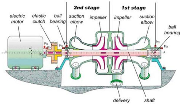
Figure 1. Cross section through the storage pump
