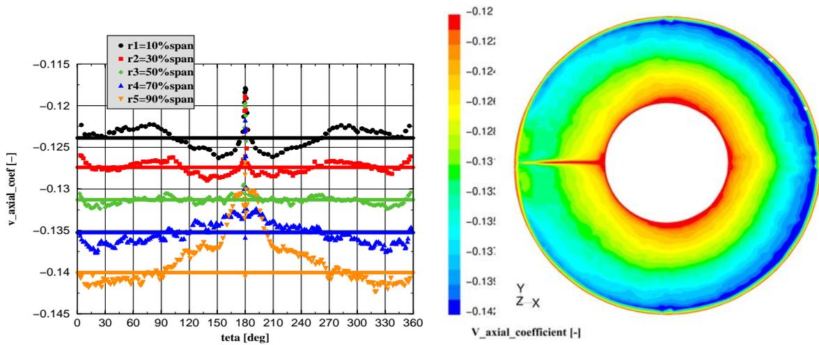
Figure 8. Axial velocity coefficient profile for the outlet section of the suction domain.
