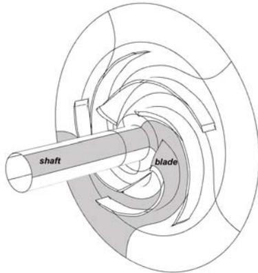
Figure 2. Isometric view of the storage pump impeller
