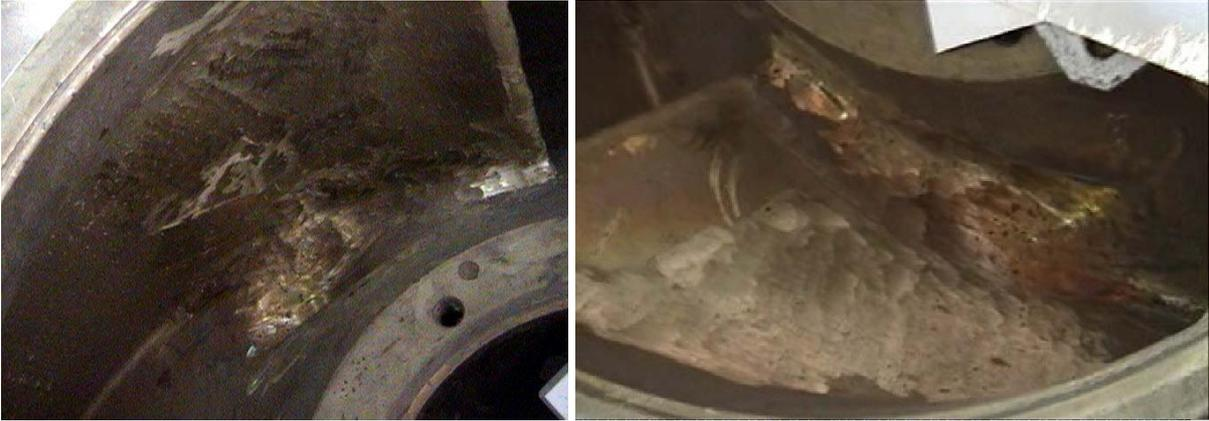
Figure 13. Cavitation erosion on the impeller blades is displaced at the junction between suction side and crown. The numerical result are in good agreement with experimental observations.
