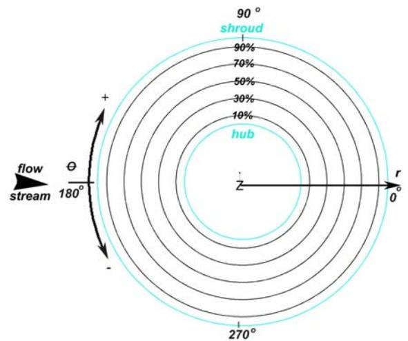
Figure 7. Coordinate system on the outlet section of the suction computational domain.
