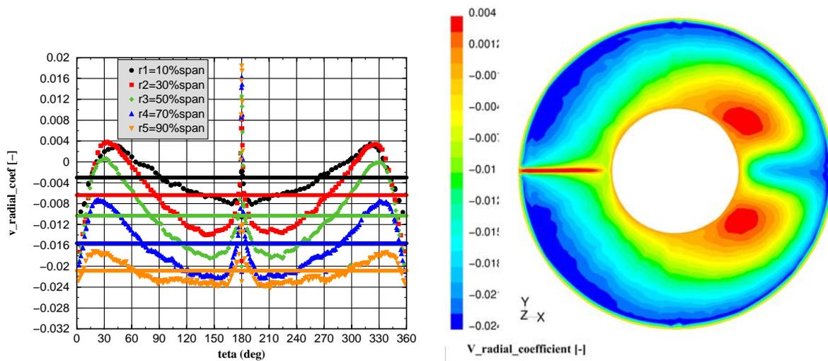
Figure 9. Radial velocity coefficient profile for the outlet section of the suction domain.
