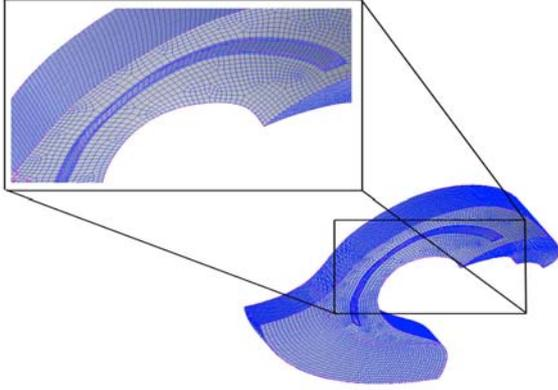
Figure 6. Mesh generated on the 3D computational domain of the inter-blade channel
