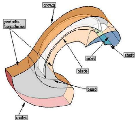
Figure 4. Isometric view of the inter-blade channel of the impeller
