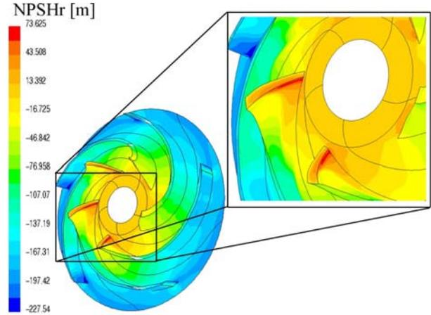
Figure 12.  $NPSH_r$  distribution on the blades for mixed velocity distribution imposed on the inlet of the impeller
