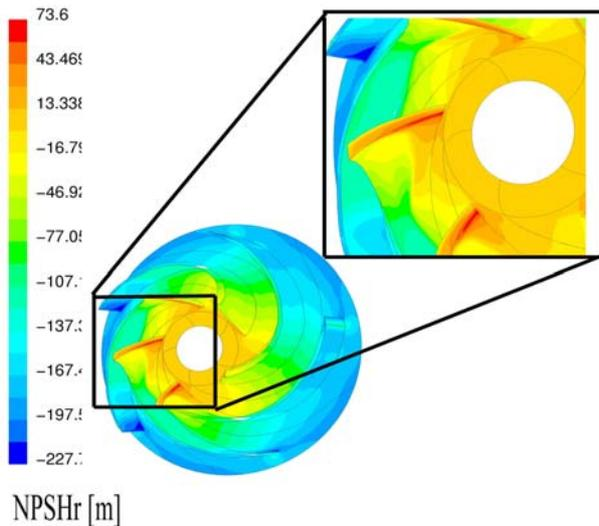
Figure 11.  $NPSH_r$  distribution on the blades for uniform velocity distribution imposed on the inlet of the impeller
