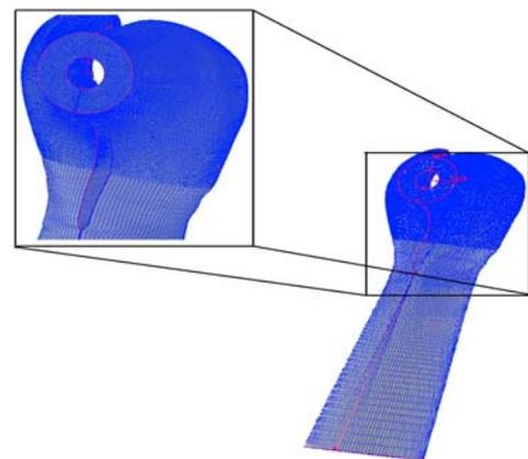
Figure 5. Mesh generated on the 3D computational domain of the pump suction
