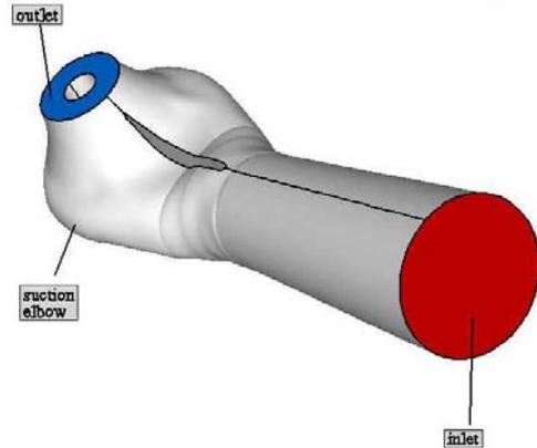
Figure 3. Isometric view of the suction domain
