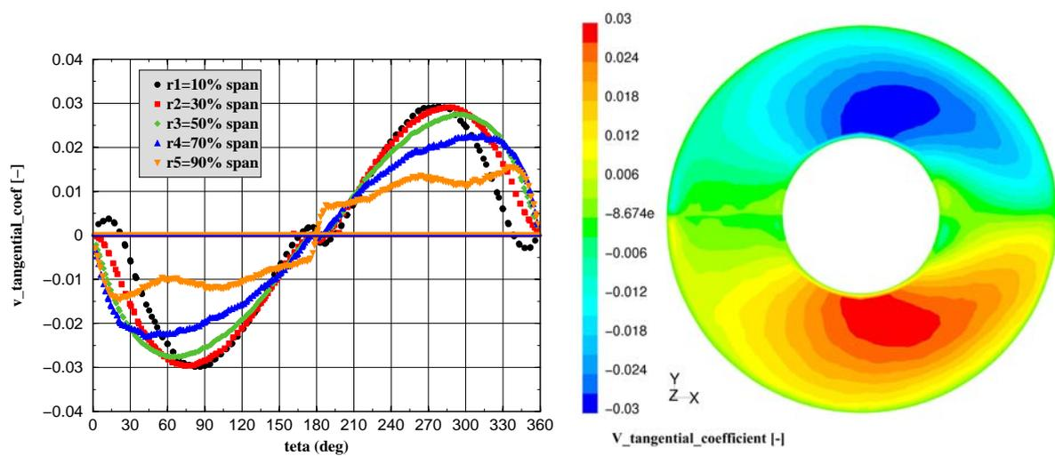
Figure 10. Tangential velocity coefficient profile for the outlet section of the suction domain.
