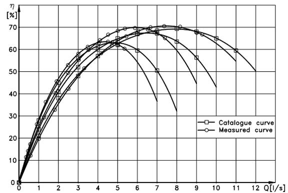
Figure 5. Pump efficiency vs. flow rate, measured and given by the pump producer
