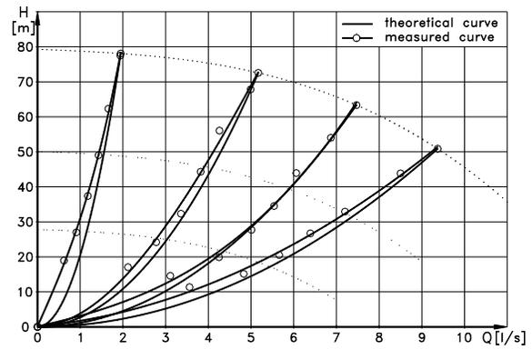
Figure 7. The pipe network operation characteristic measured and calculated
