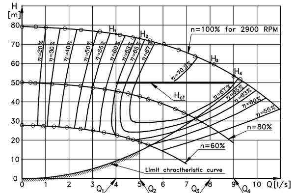
Figure 9. The characteristic curves of the pump
