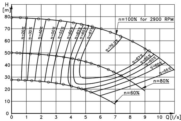
Figure 6. The pump operation characteristic according to measured data with the thermodynamic method
