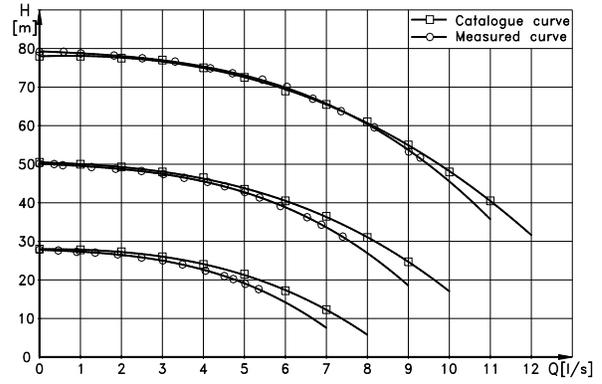
Figure 4. Pumping head vs. flow rate, measured and given by the pump producer
