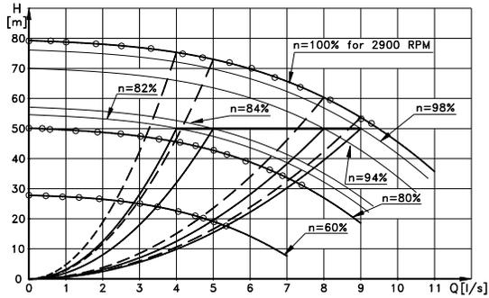
Fig. 10 The exploitation domains and the limit hydraulic characteristics
