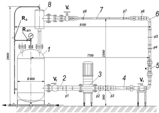
Figure 1. Multifunctional installation loop facility (without the measuring instruments)
