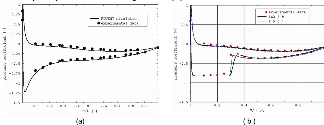
Figure 5. Pressure coefficient distribution of the different turbulence intensity for NACA 0009 hydrofoil at no-cavitating condition (a) and (b) cavitation number = 0.81 .
