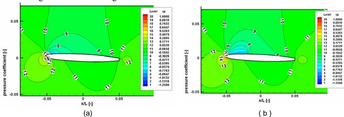
Figure 4. Pressure coefficient distribution on the NACA 0009 hydrofoil at 2,5 degree angle of attack. a) No cavitation; b) cavitation number 0.81.
