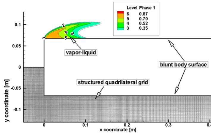
Figure 1. Predicted liquid volume fraction and surface pressure contours, selected streamlines and computational grid for a blunt-body, at cavitation number  $\sigma = 0.5$ .
