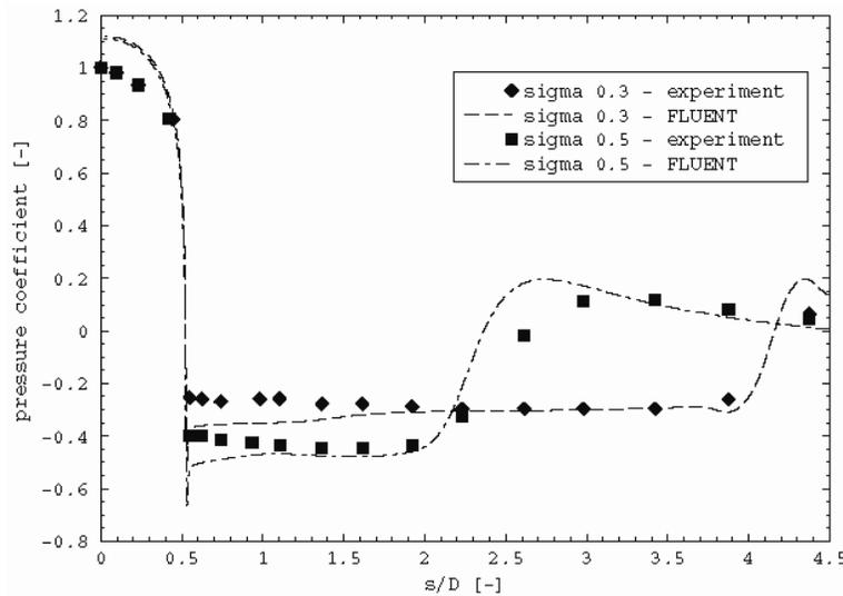
Figure 2. Comparison of predicted and measured surface pressure distributions at several cavitation numbers for a blunt-body.
