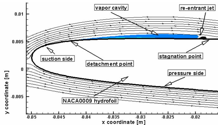
Figure 3. Computed total volume fractions distributions and selected streamlines for NACA 0009 hydrofoil at cavitation number = 0.81.
