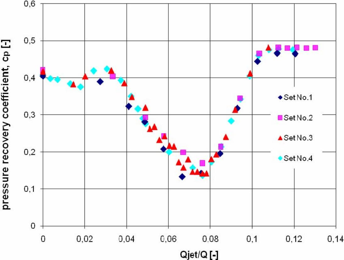
**Fig. 7:** Pressure recovery coefficient against ratio between axial jet control discharge ( $Q_{jet}$ ) and main flow discharge ( $Q$ ).
