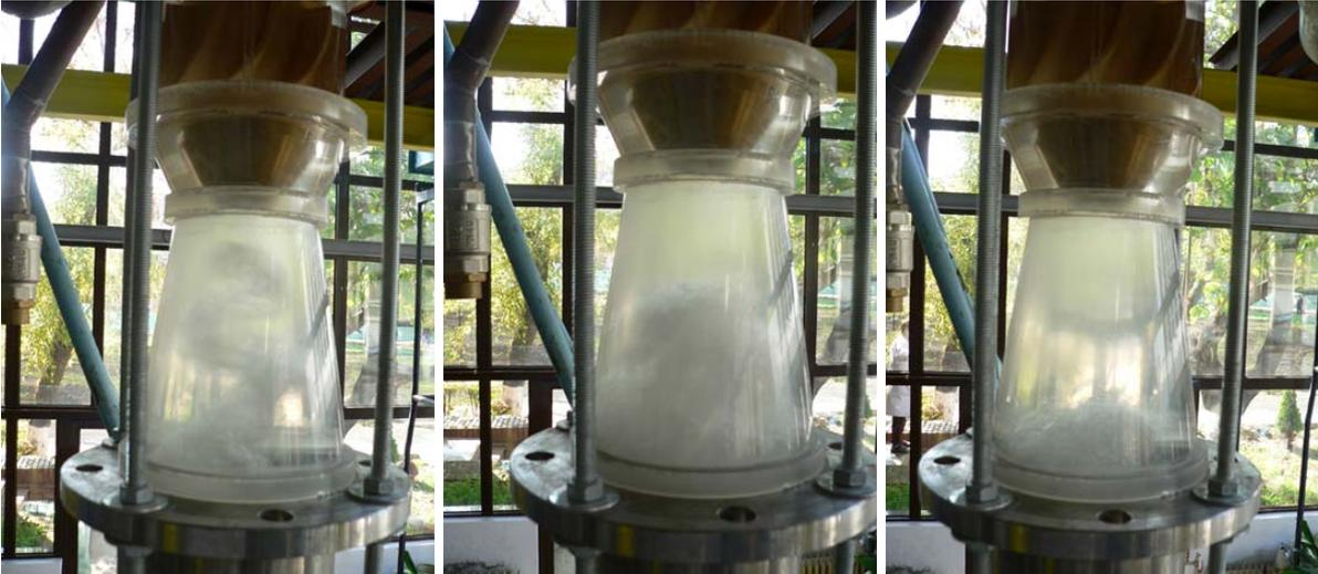
a) no jet control                      b) with axial control jet discharge at two different values
