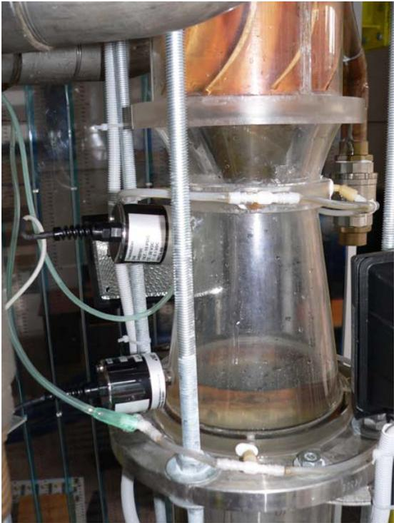
**Fig. 5: Pressure transducers mounted on the cone wall**
