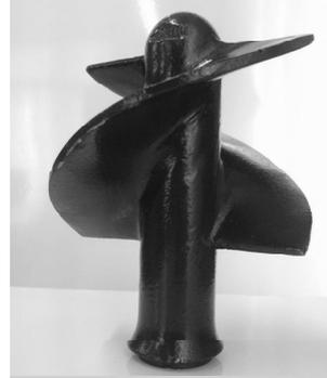
Figure 3. The inducer investigated experimental and numerical
