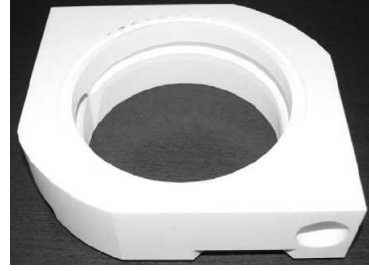
Figure 11 Spiral case made by rapid-prototyping machine.
