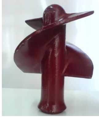
Figure 3. The inducer investigated experimental and numerical
