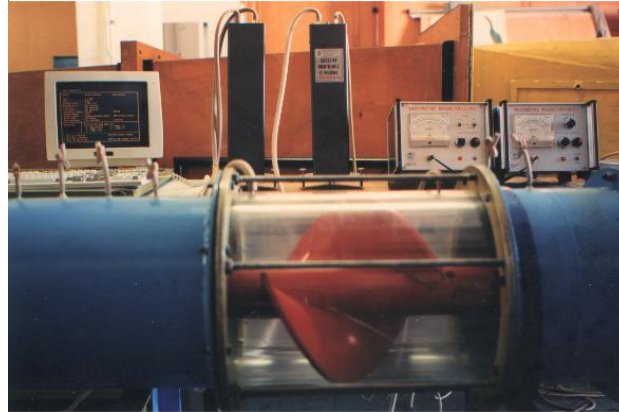
Figure 6. Test rig for pressure measurement on the blade of an inducer
