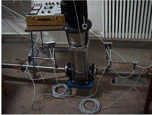
Figure 2. Connection of the pressure and temperature probes for the pump testing
