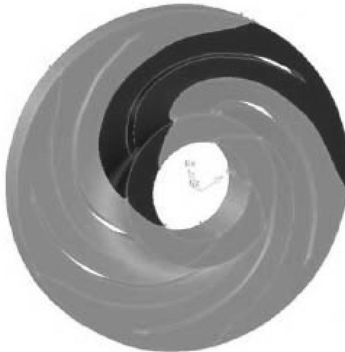
*Fig.1 Impeller of the storage pump with highlighted inter blade channel*
