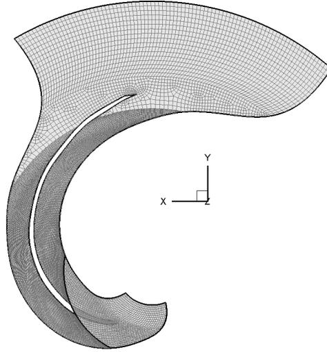
Fig.2 Mesh generated on the 3D computational domain of the inter-blade channel
