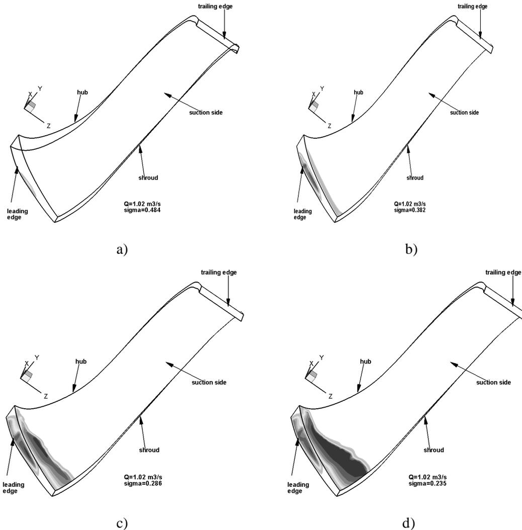
*Fig.5 Distribution of the volume of vapour on the suction side of the blade for different cavitation numbers*
