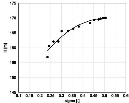
Fig.6 Pumping head drop due to cavitation
