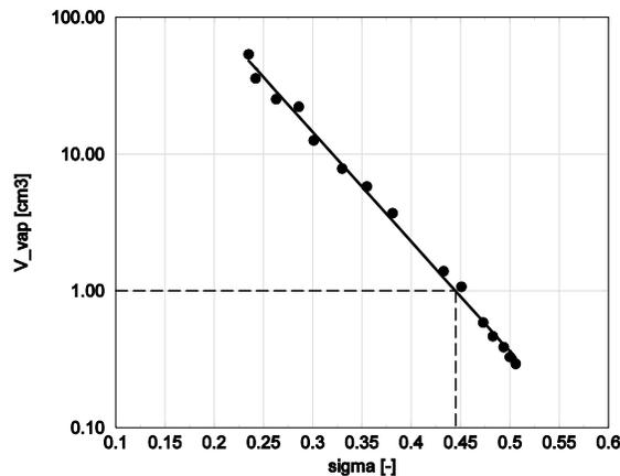
Fig.4 Variation of the volume of vapour against the cavitation number for best efficiency point
