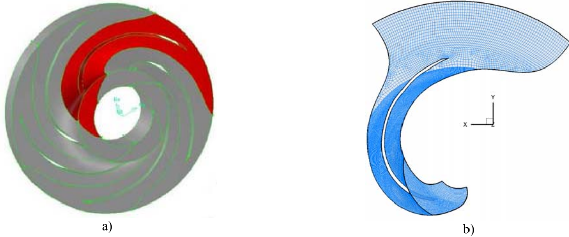
Fig. 2 a) Impeller of the storage pump with highlighted inter blade channel b) Mesh generated on the 3D computational domain of the inter-blade channel
